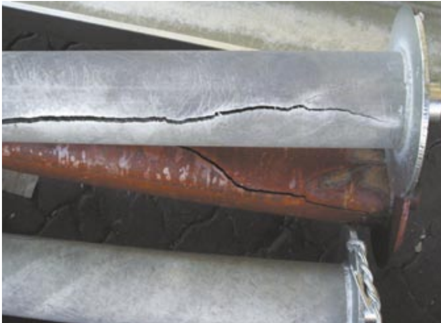
Spectacular hydrogen embrittlement failure of high strength quenched and tempered (1200 MPa) steel drill pipes. Note ungalvanized failed pipe as embrittlement occurs in the pickling process.
