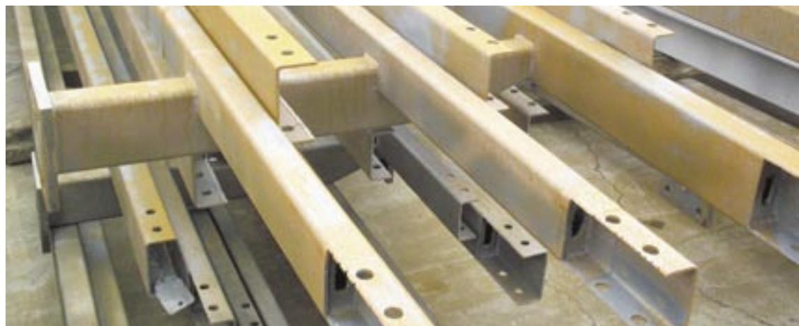
These refurbished bridge rails have been Sa Class 2 abrasive blasted prior to hot dip galvanizing.
