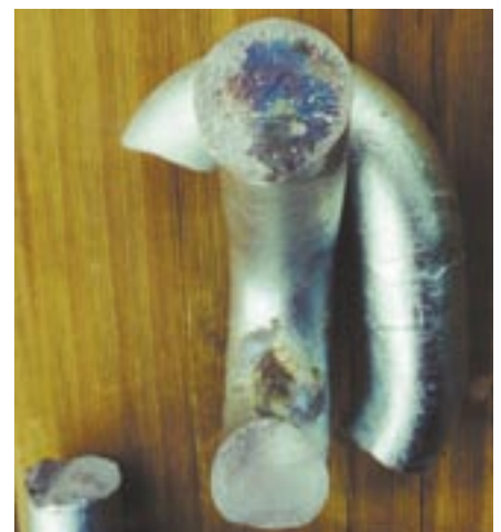
This section of chain fractured after galvanizing. It was found to be high tensile Herculloy-type chain (1200 MPa yield) rather than standard Grade 80 that was specified. The failure is a result of hydrogen embrittlement.
