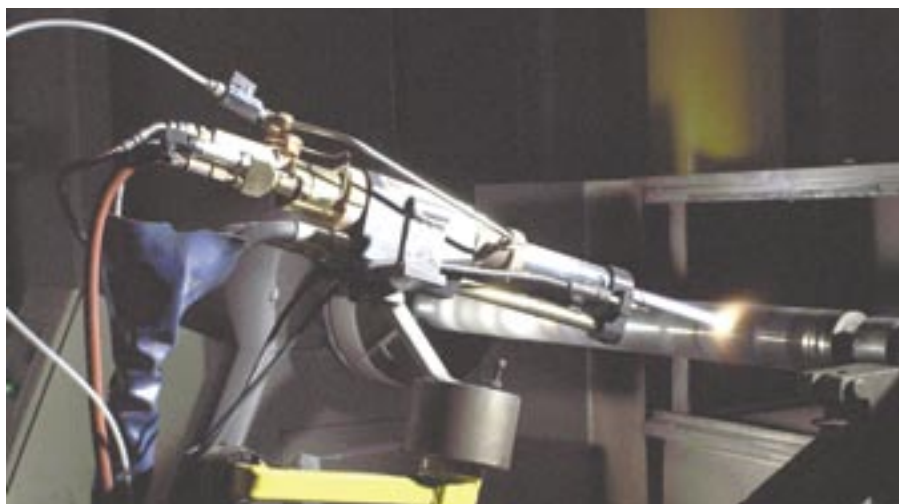
Metal spraying technology can be used with a wide range of metals for other than corrosion prevention. This application is building up a worn area on a shaft with wear resistant material.
