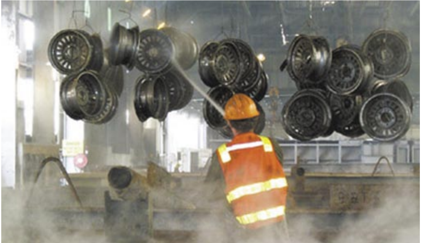
Chemical pretreatment facilitates surface preparation for complex shapes, with costs almost an order of magnitude lower than mechanical pretreatment processes.
