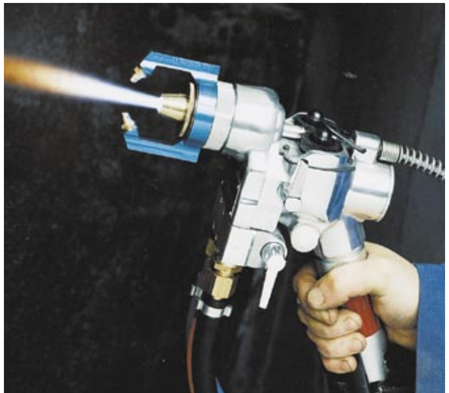
Flamespray MK 73 gun uses a gas flame to melt the metal feed wire.
