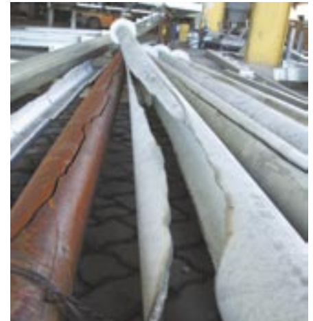
Spectacular hydrogen embrittlement failure of high strength quenched and tempered (1200 MPa) steel drill pipes. Note ungalvanized failed pipe as embrittlement occurs in the pickling process.
